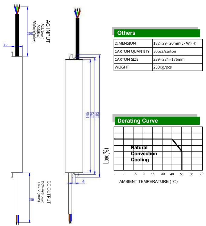
Cable Model of input: H03VV-F 3G0.75mm<sup>2</sup>
